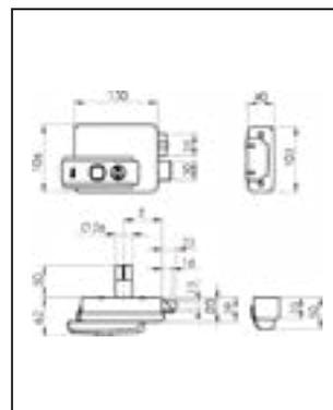
**ISEO****ELETTROSERRATURE DA APPLICARE SERIE ELETTRICA 500**
